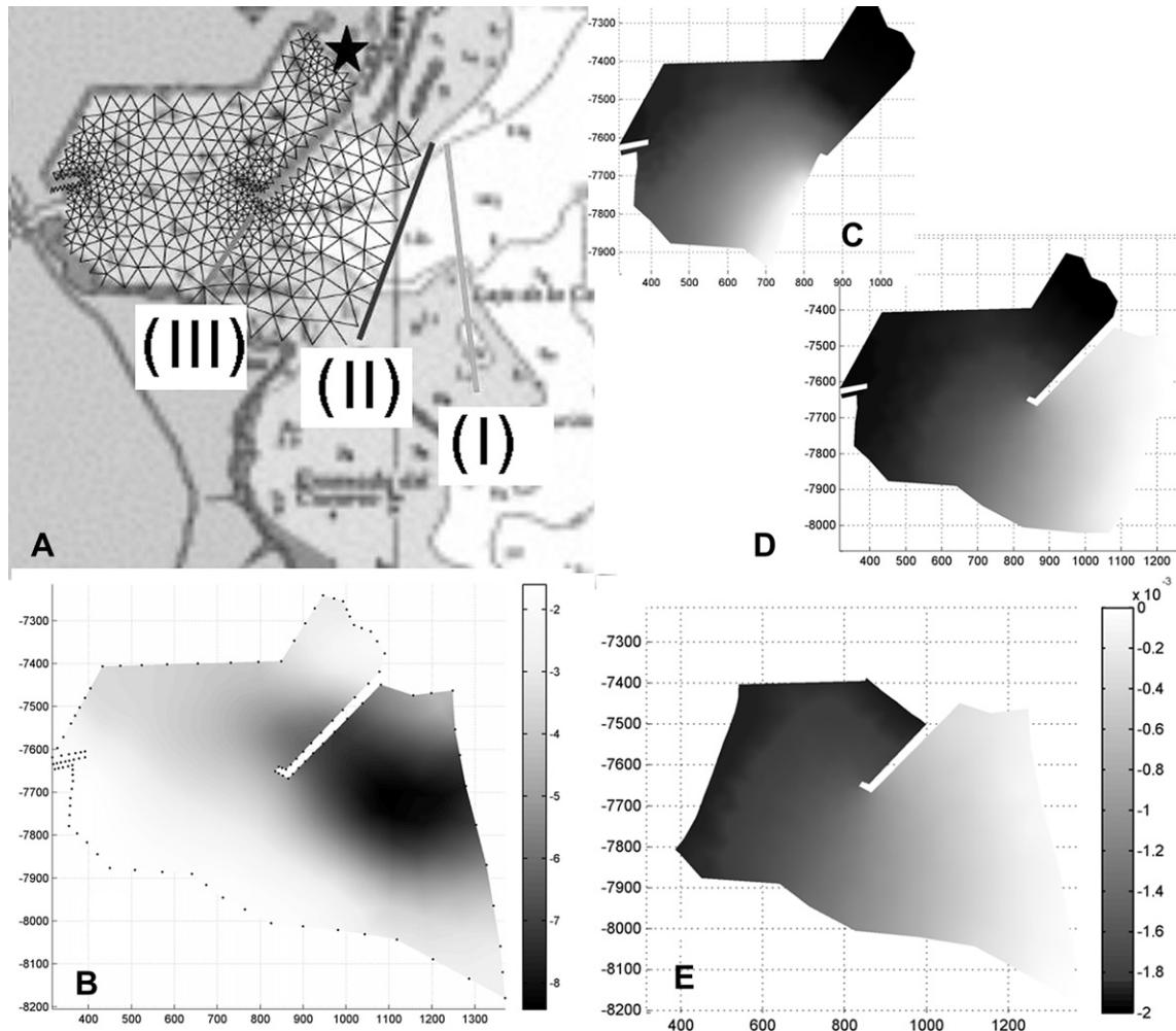
**Fig. 7.** (A) The same as Fig. 5 for Algeciras. (C), (D) and (E) are fundamental mode with period 8.7, 12.4 and 13.7 min for open boundary at III, II and I respectively.
