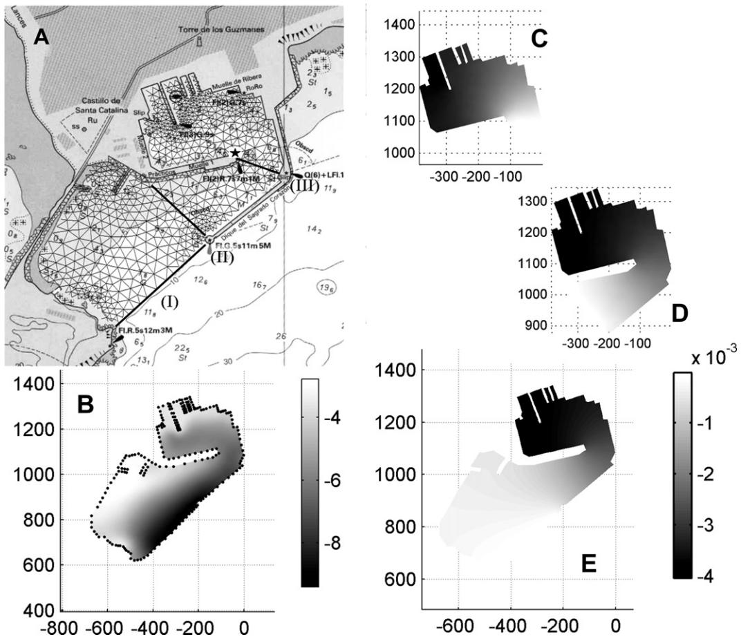
**Fig. 6.** The same as Fig. 5 for Tarifa. Lines I, II and III indicate three choices of the open boundary. (C), (D) and (E) are spatial pattern of the fundamental mode with period of 4.3, 7.0 and 7.8 min for open boundary at III, II and I respectively.
