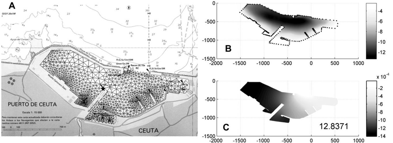
**Fig. 5.** (A) Grid of the numerical model at Ceuta. The star marks the position of the tide-gauge. (B) Bathymetry used in the numerical model. (C) Spatial pattern of the fundamental mode (period of 12.8 min). Axis units are meters from an arbitrary origin. Contours in panel C are meters  $\times 10^{-4}$ . Notice that these units are somewhat arbitrary due to the linearity of Eq. (4).
